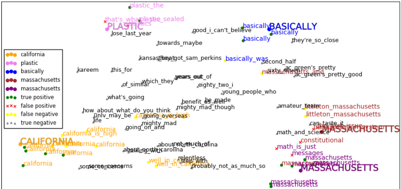
Figure 4: Embeddings of queries and their top hits, visualized in two dimensions using t-SNE [31]. Queries are shown in capital letters. The top several hits for each query are shown in the same color as the query. Random segments from the search collection and their associated transcriptions are shown in gray.
