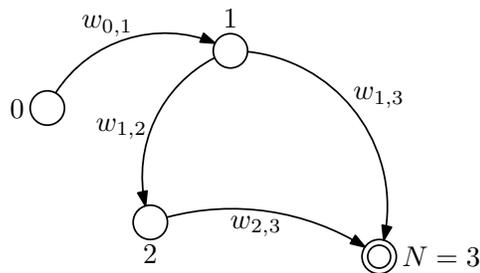
We want to find the path through such a graph that gives the lowest cost when adding up all the weights on that path. Let us define  $\alpha_i$  as the cost of the best path up to node  $i$ . I.e.,  $\alpha_i$  is the sum of the weights on the shortest path from node 0 to node  $i$ . We will define it more formally in just a little bit. Given this definition, we can find the shortest path by applying the following *forward* recursive steps:
