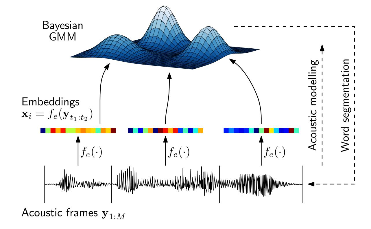
BES-GMM uses Gibbs sampling for joint segmentation and clustering. Downsampling is used as embedding function  $f_e(\cdot)$  for ES-KMeans and BES-GMM. ES-KMeans results in the limit from BES-GMM when the variance  $\rightarrow 0$ .
